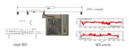
between electrodes a few kilometers or tens of kilometers apart (large dipoles).
